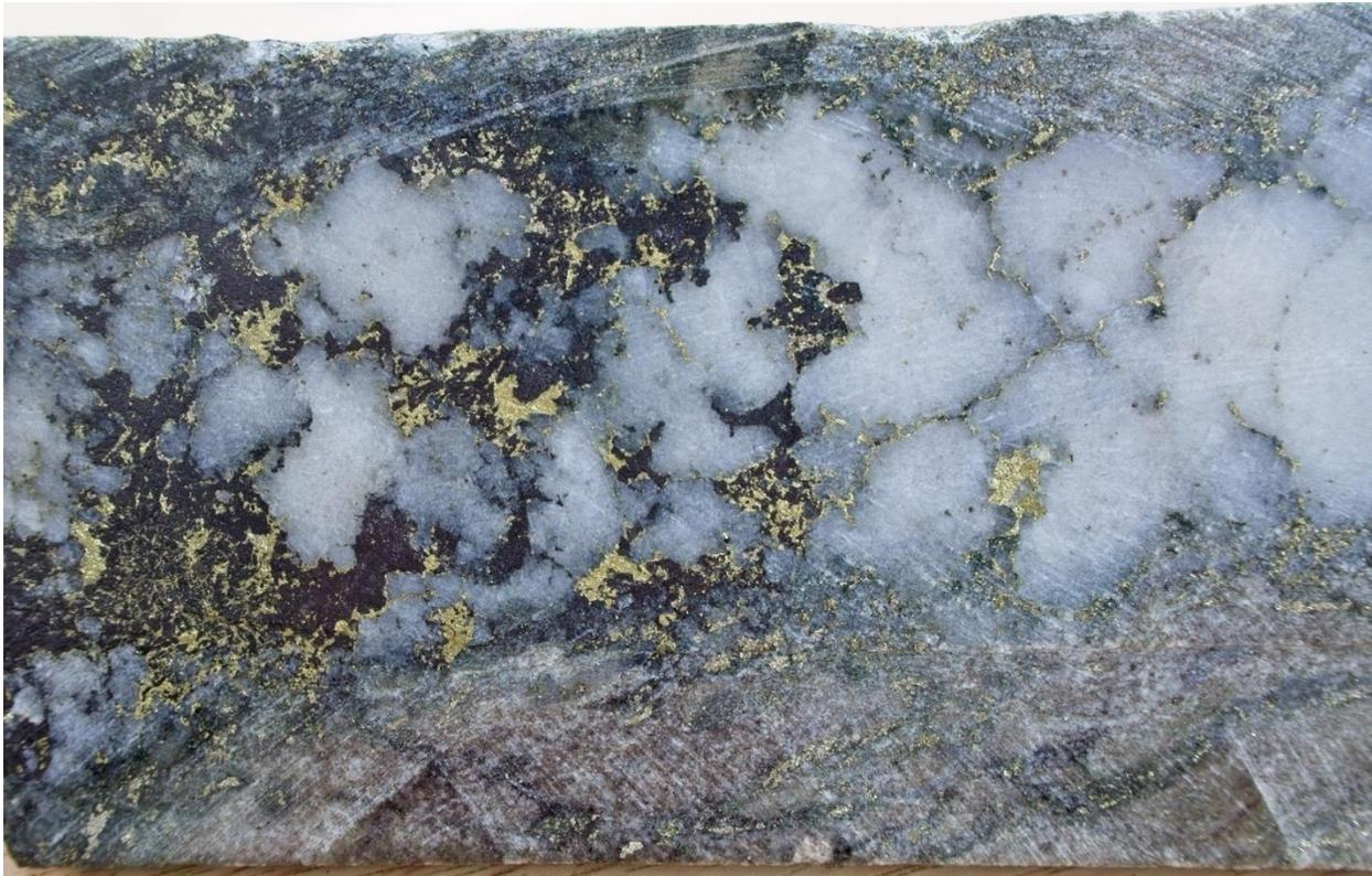
**Image 2.** ELID022, 209.2 m from a sample interval reporting **1.43% Cu, 0.037% Mo, 9.5 g/t Ag**. A chalcopyrite-pyrite vein in potassic-altered feldspathic arenite containing pervasive secondary biotite. Chalcopyrite is introduced by sulfide veins like the one shown here and quartz-pyrite-chalcopyrite-molybdenite veinlets (A veins). Core is HQ diameter (63.5 mm).
